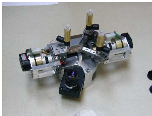
Figure 8: Servo-controlled multi-functional gripper with two degrees of freedom and three grasping elements (“fingers”). Also shown are selected examples of grasping configurations for different objects.
